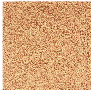
PEBBLE BEACH 1.5 aggregate size to produce a uniform medium sand finish (NOTE: this texture used to be called Pebble Beach Fine)
