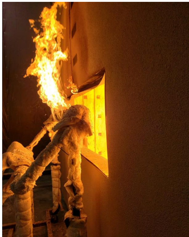
Figure 1. Diamond Wall during NFPA 285 noncombustible fire test.
